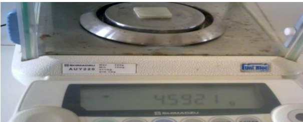
Fig. 14(a) Weight of the specimen (b) Specimen in muffle furnace.
